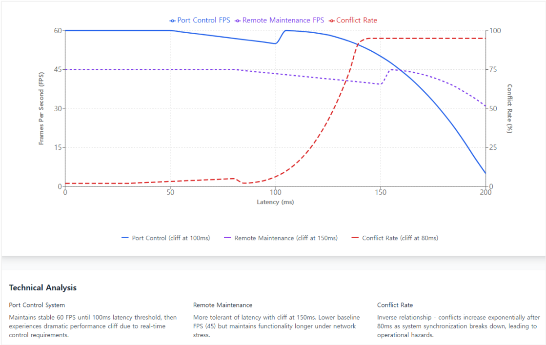
Figure 5.2: Performance Degradation Curves by Use Case (Conceptual graph with latency (0-200ms) on the X-axis and performance metrics (FPS, conflict rate %) on the Y-axis. Separate curves for the port control FPS and remote maintenance FPS and conflict rate are shown, each exhibiting a 'cliff' shape where the slope steepens dramatically after a certain latency.)
